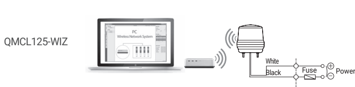
Ethernet connection via Gateway
